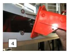
tension." (force required to collapse goal) The tension can be set anywhere from 170 lbs. to 230 lbs. Simply insert a 5/32" T handle hex wrench into the hole located at the bottom of the cover plate. Turn the hex wrench clockwise to increase tension or counterclockwise to decrease tension. The wrench can be purchased at most tool supply stores.
